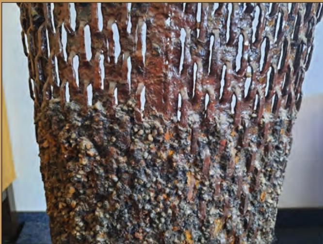
Figure 4. The upper half of this low open area bridge slotted pipe was rehabilitated with the high-pressure impulse process.
